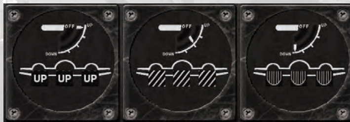
The WING FLAP Indicator positions (UP, HALF, DOWN).
