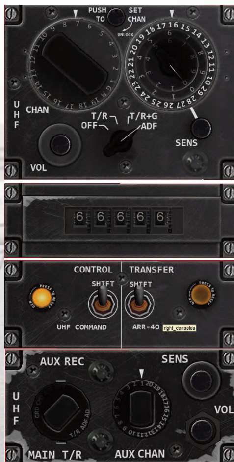
T-2A (T-2J-1-S) Communications Panel: AN/ARC 27A UHF Set AN/ARN 21 Radio Navigation (TACAN) AN/ARR 40 UHF Aux Set
